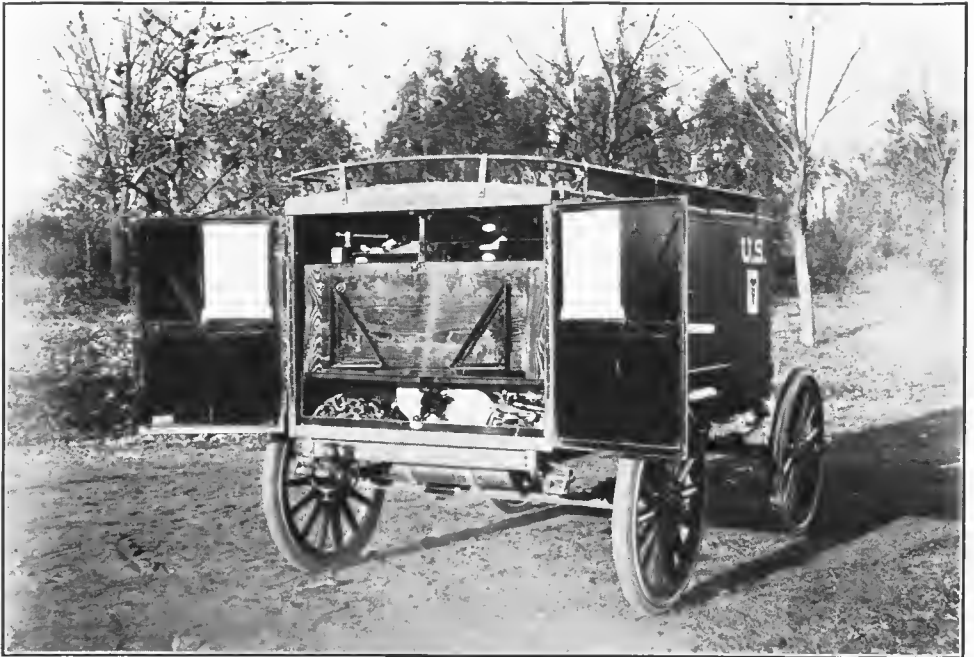
FIG. 30.—Spare parts trailer, rear view
