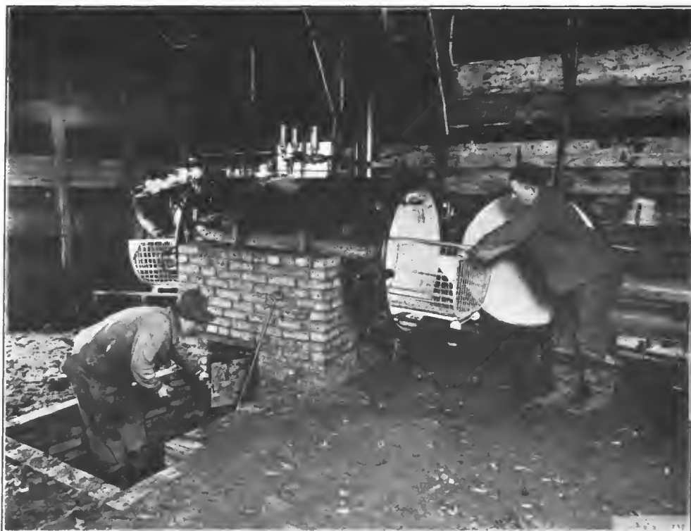
FIG. 125.—Stationary, furnace-heater type, Thresh disinfector for base hospital use, A. E. F.
