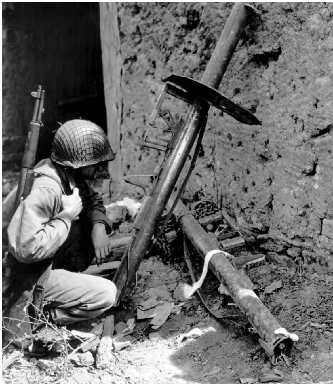
AN INFANTRYMAN ARMED WITH AN M1 RIFLE looks at two German rocket launchers left behind by the enemy (8.8-cm. Rakettenpanzerbuchse ). The German weapon was of larger caliber and was heavier than the U. S. rocket launcher but similar in appearance and operation.
