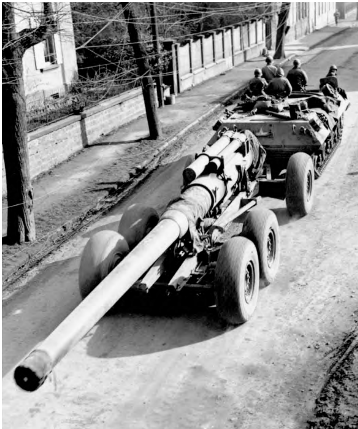
TUBE AND RECOIL MECHANISM OF AN 8-INCH GUN M1 on the way to the front.
