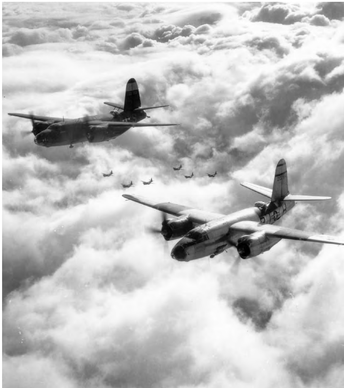
MARTIN B-26'S RETURNING FROM A MISSION along the German border in support of the Third Army's ground attack. The medium bomber in the upper foreground of the above picture had operated in the ETO for some time, as is shown by the dark-painted fuselage. The plane in the lower foreground has an unpainted fuselage which enabled it to attain higher speeds.
