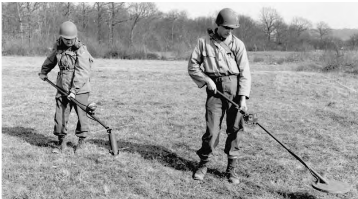
TWO TYPES OF MINE DETECTORS. At left, AN/PRS-1 type; at right, SCR 625 (top). Mine detectors were developed by the Signal Corps primarily for use by Engineer troops. Signal Corps repairmen splicing wires of an underground cable which was damaged by artillery fire (bottom).
