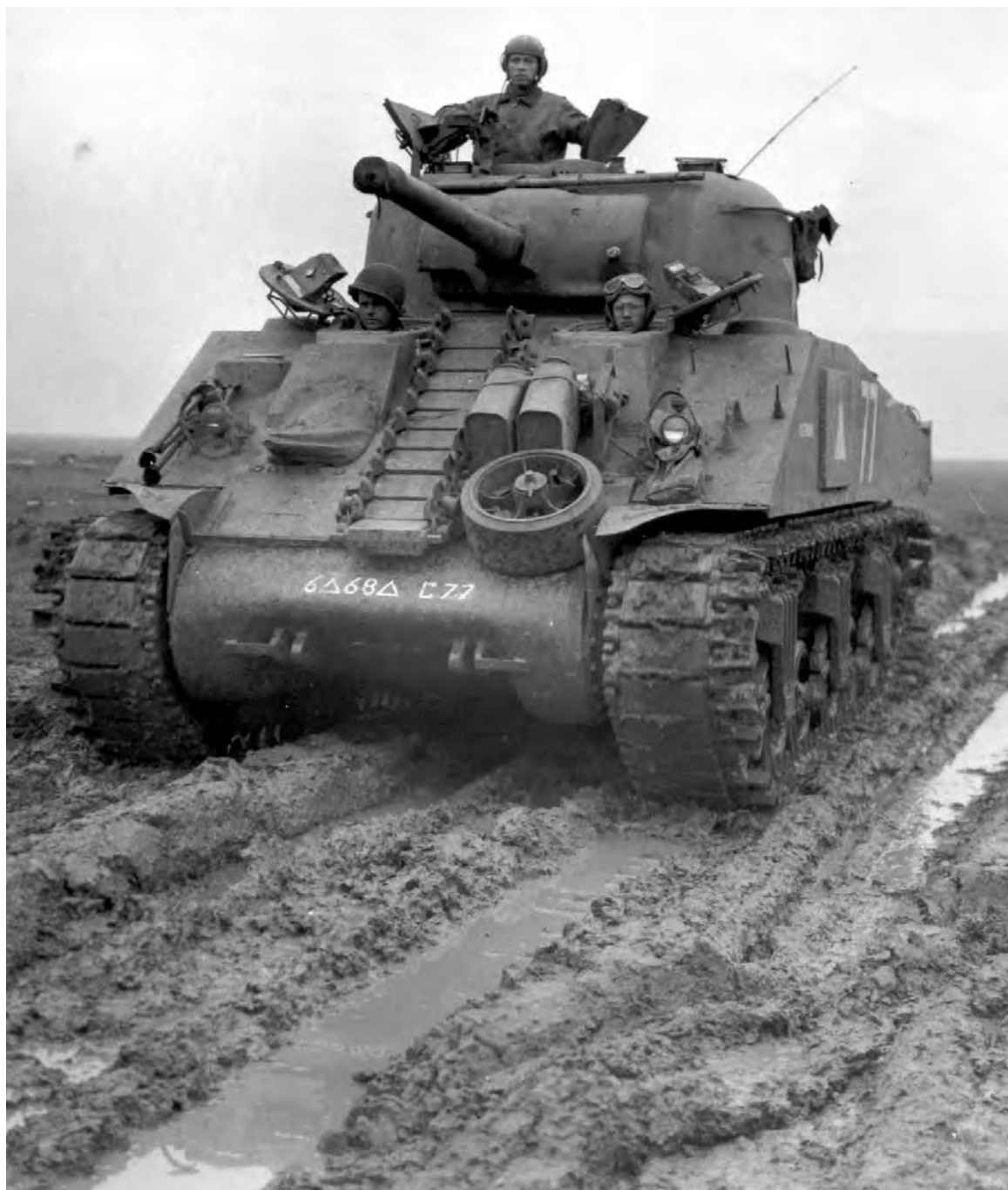
AN M4A3 MEDIUM TANK fitted with track extensions maneuvering through soupy ground. Track extensions were so devised as to give better flotation and traction through the November mud.
