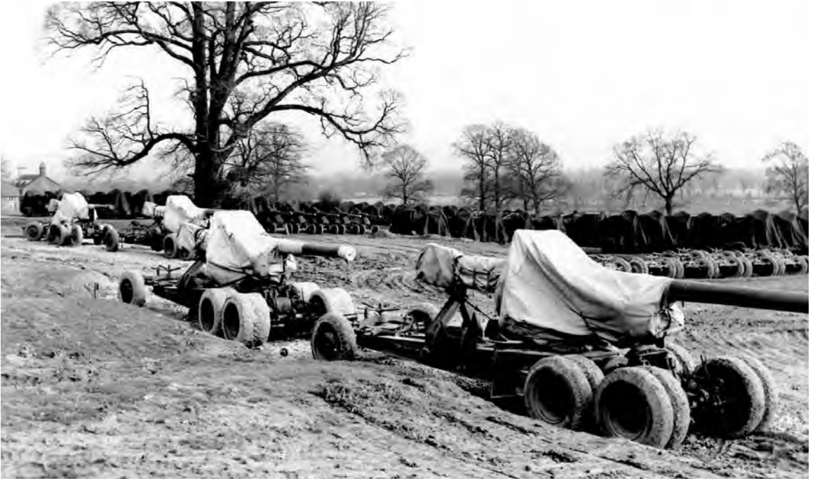
155-MM. GUNS AND 105-MM. HOWITZERS (top and bottom respectively) stored in England, 1944. After about 2,250 rounds had been fired, the barrel of the 155-mm. gun had to be replaced; in howitzers the number of rounds was higher.
