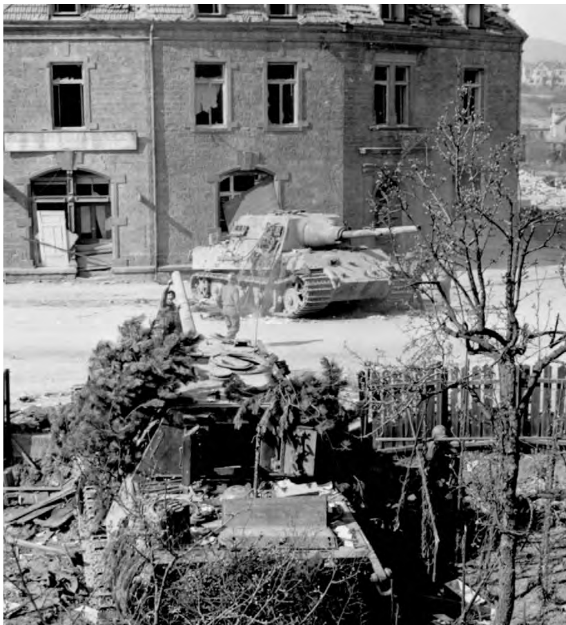
TWO KNOCKED-OUT GERMAN SELF-PROPELLED GUNS ( Pz. Jaeg. Tiger with 12.8-cm. PJK 44 ). This vehicle, called a Jaegdtiger , was the most formidable self-propelled antitank gun used by the Germans during the war. It consisted of a 12.8-cm. PJK 44 (L/55) (less muzzle brake) mounted on a Tiger B chassis. The gun could penetrate 6 to 8 inches of armor at 1,000 yards. Weight of the vehicle was 77 tons.
