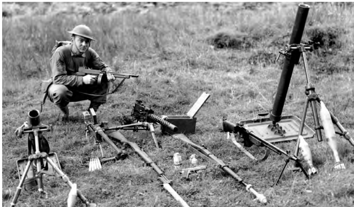
INFANTRYMAN WITH WEAPONS. Soldier is holding a .45-caliber Thompson sub-machine gun M1928A1; from left to right are: 60-mm. mortar M2, British antitank gun, .30-caliber U. S. rifle M1 with bayonet M1 attached, .30-caliber Browning machine gun M1919A4, hand grenades, .45-caliber automatic pistol M1911A1, .30-caliber U. S. rifle M1903 with grenade launcher M1 attached, .30-caliber Browning automatic rifle M1913A2, and 81-mm. mortar M1 (top). Infantryman has just completed an obstacle course (bottom).
