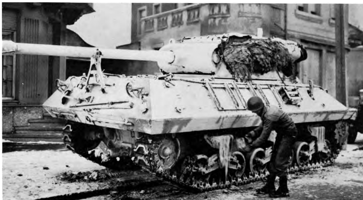
CAMOUFLAGED LIGHT ARMORED GAR M8 and one that has not been painted white, showing the effectiveness of snow camouflaging (top). A crew member of a 90-mm. gun motor carriage M36 throwing paint on the bogie wheels after painting the vehicle (bottom). Tanks, vehicles, and guns were camouflaged with white paint.
