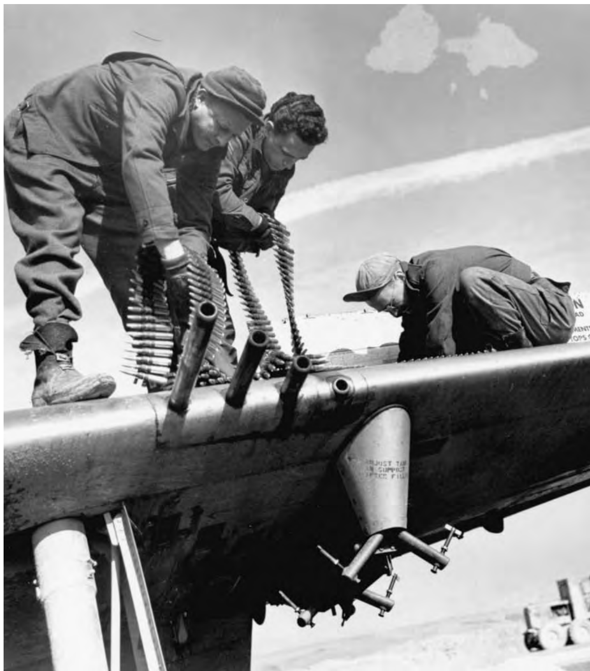
LOADING .50-CALIBER AMMUNITION into the wing of a P-47 Thunderbolt fighter plane. On 22 February one of the greatest aerial operations of the war was carried out by nearly 9,000 aircraft taking off from bases in England, France, the Netherlands, Belgium, and Italy. The targets, the German transportation facilities, covered an area of over a quarter of a million square miles.
