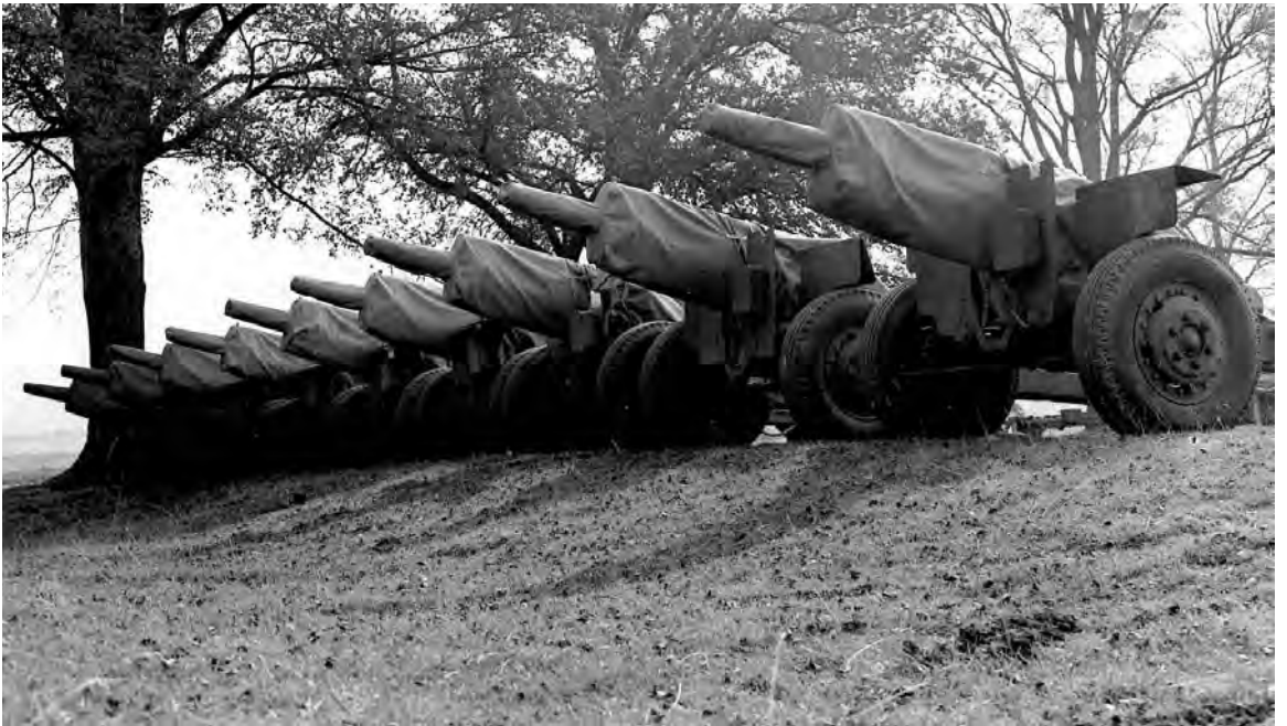
155-MM. GUNS AND 105-MM. HOWITZERS (top and bottom respectively) stored in England, 1944. After about 2,250 rounds had been fired, the barrel of the 155-mm. gun had to be replaced; in howitzers the number of rounds was higher.
