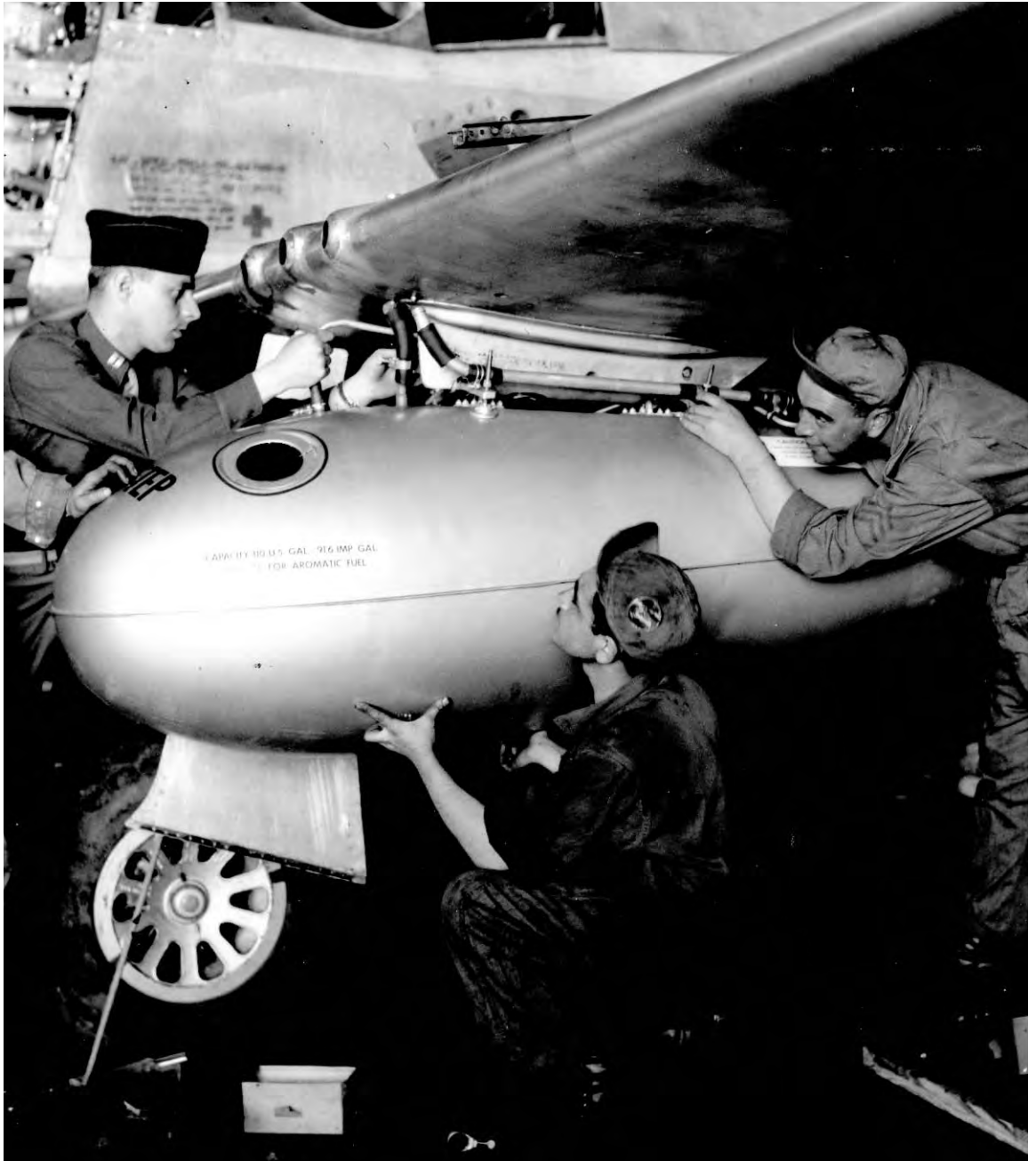
MEN OF A SERVICE SQUADRON SALVAGING A FUEL TANK from the wing of a P-51. These tanks helped to make the bomber escort planes into long-range planes which gave fighter protection to the heavy bombers. The tanks, the fuel from which was consumed first, were dropped when empty and the plane then used gasoline from its permanent tanks.
