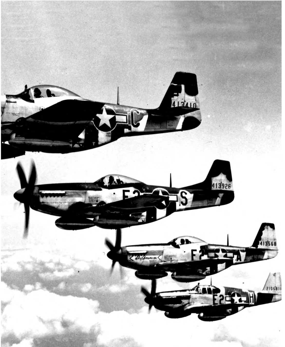
P-51'S IN FORMATION. Each plane in this formation has two wing tanks attached.
