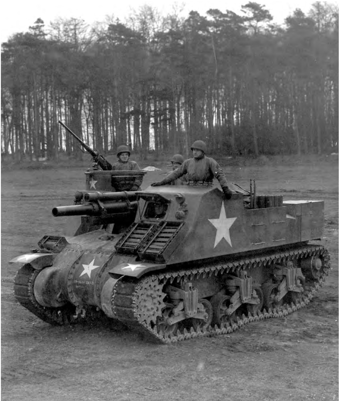
A 105-MM. HOWITZER MOTOR CARRIAGE M7 on maneuvers in England, March 1943. This was an open-top, lightly armored vehicle and was the principal artillery weapon of an armored division.
