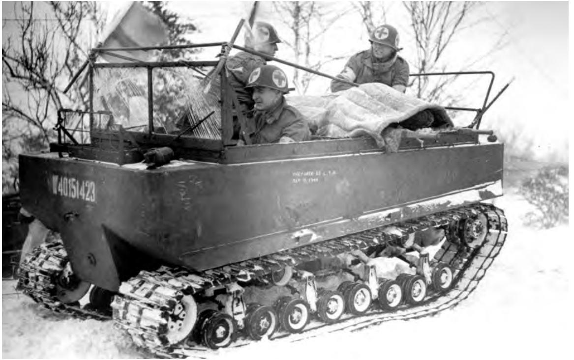
WOUNDED SOLDIERS BEING EVACUATED in tracked vehicles during the winter months. Cargo carrier M29 (top) ; half-track personnel carrier M3 (bottom).
