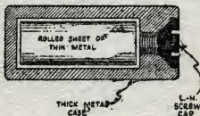
SECTIONAL DETAIL OF METAL CYLINDER, FOUND ON MOORS (1 1/4" X 3" FULL SIZE)
