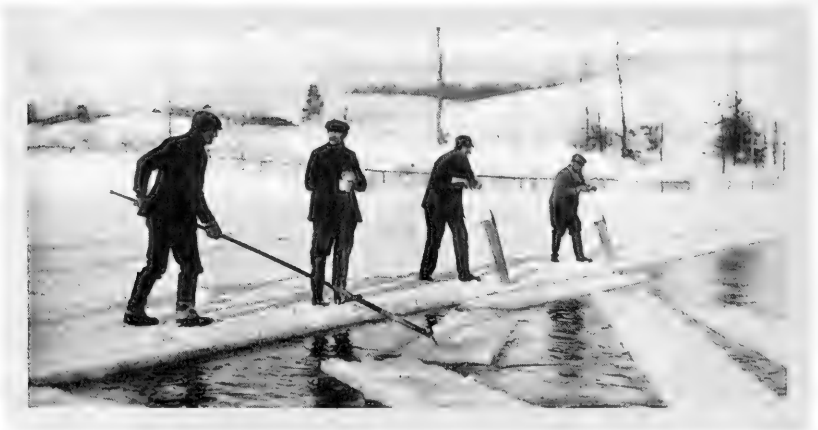
SEPARATING LONG SLABS OF ICE WHICH HAVE BEEN MARKED INTO SQUARES BY PLOUGHS.
