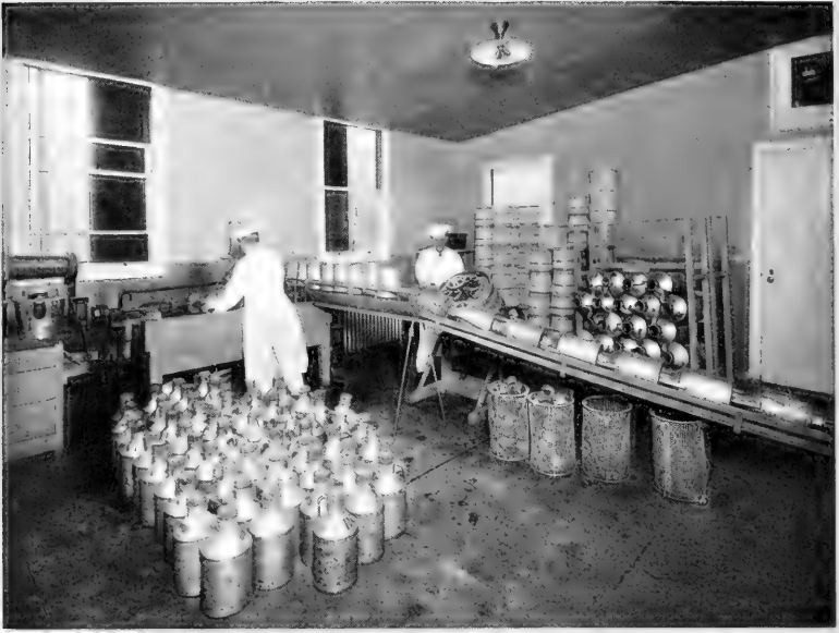
WASHING CANS AND STOPPERS WITH HOT WATER AND STEAM JET.
