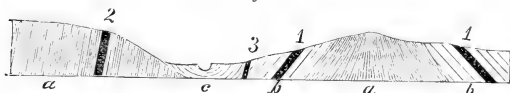
Fig. 13.—Ideal Section, showing the general relations of the Iron Ores of the East River of Pictou.
