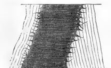
Fig. 65.—Relation of the "Albert Coal" to the containing beds, as seen near the shaft of the mine.
