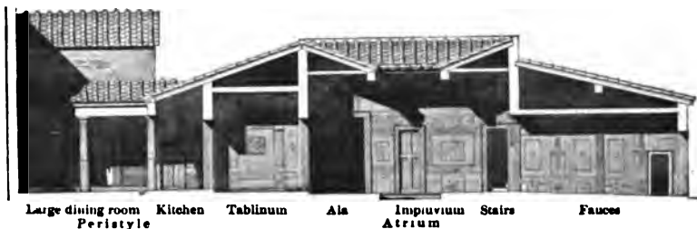
Fig. 21. Section through the house of the Tragic Poet, restored. Mau, Pompeii , fig. 154, p. 304, ed. 1900 (Mau-Kelsey, p. 316, ed. 1902).
