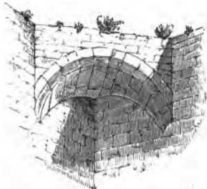
Squinch, Canon's Ashby, Northamptonshire.
