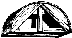
Centering of a round-headed arch.
