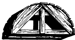
Centering of a round-headed arch.
