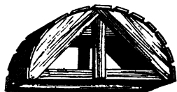
Centering of a round-headed arch.
