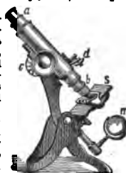
Microscope. a Eyepiece; b Objective; c Rack and Pinion for coarse adjustment of focus; d Screw for fine adjustment; e Mirror; f Stage.
