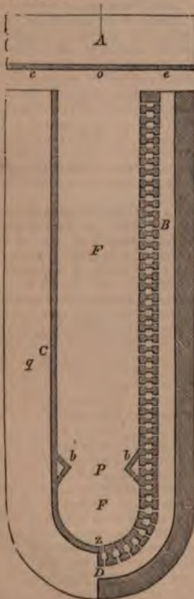
A is the boundary wall at the aphesis, 77 feet deep. B C the sides, and D the semicircular end, of the same depth as A; F F the area, including the σφενδομή ; b b pieces of masonry jutting out into the area; e e the entrances; from o to P is the
