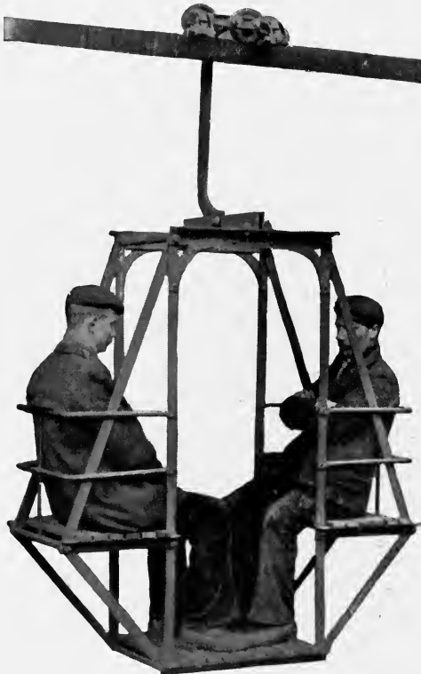
FIG. 63.—Passenger Carrier for Running-Rope System.
