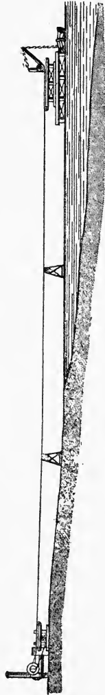
FIG. 98.—Installation of Wire Rope-Way driven by Portable Engine arranged as a Pier in New Zealand.
