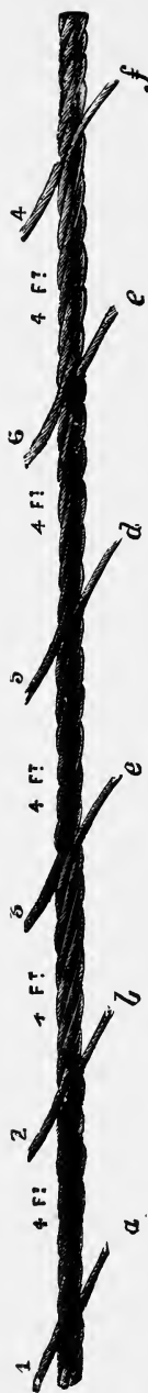
FIG. 150.—Splicing Wire Ropes: Third Operation.
