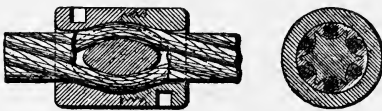
FIGS. 33 and 34.—Modified Form of Otto Knot or Carrier Collar. Longitudinal and Cross Sections.
