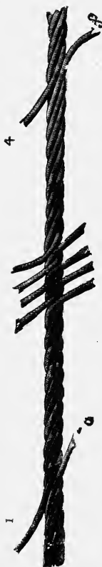
FIG. 149.—Splicing Wire Ropes: Second Operation.
