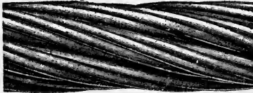
FIG. 10.—Wire Rope, Albert Lay : Appearance when New.
