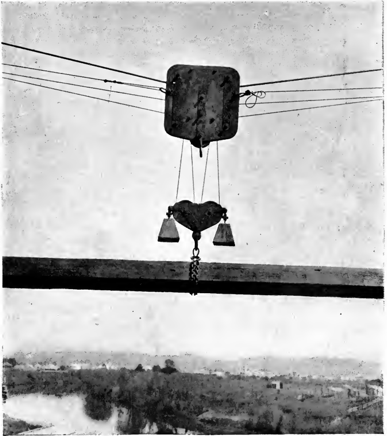
FIG. 141.—Wire Rope-Way for Hoisting and Conveying : Carrier or Running Head.
