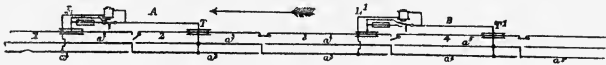
FIG. 67.—Blocking Arrangement for a Trolley Line with Minimum Interval equal to one Section of the Main Conductor.
