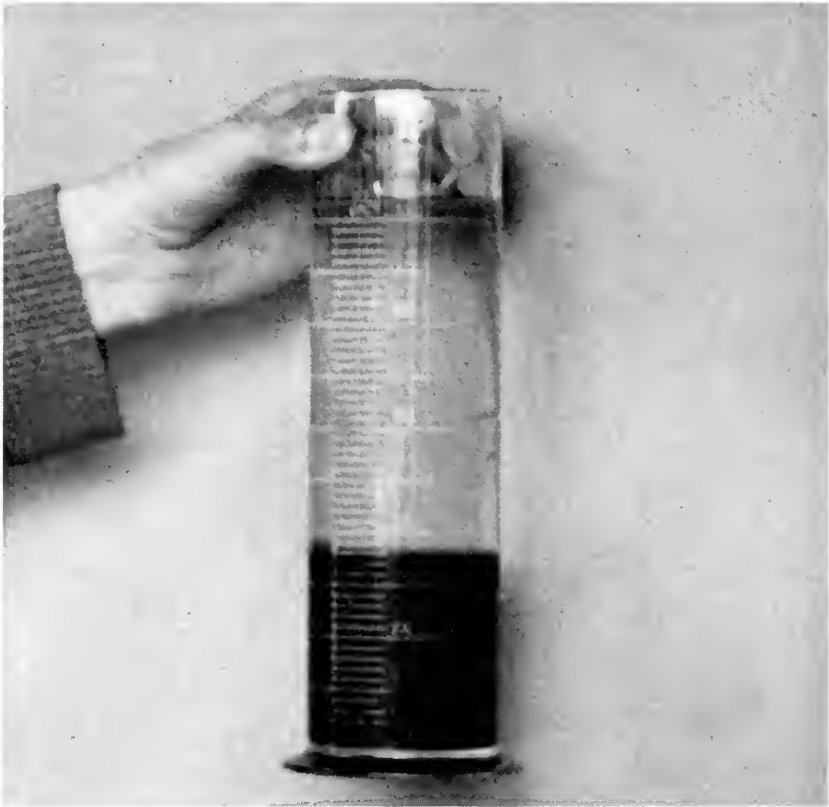
Separation of solids and supernatant after approximately 30 minutes of quiescent conditions. (Fig. 13)
