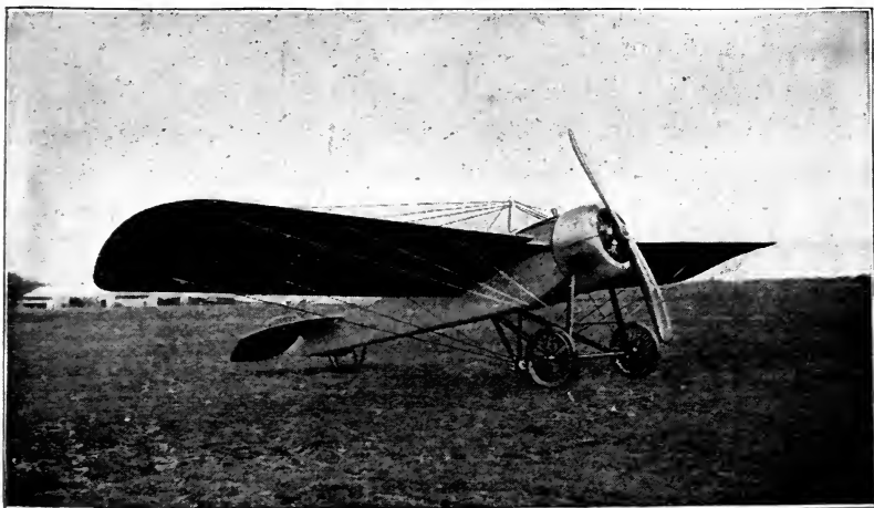
FIG. 22.—Nieuport single-seater monoplane (1914).
