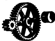
Fig. 207. Spur gearing. The pinion or small gear to the right is "shrouded."
