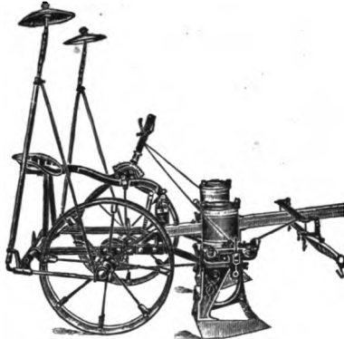
Fig. 144. A corn planter with stub shoe furrow-openers.
