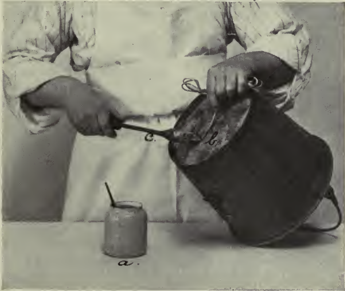
Repairing leak in water-bucket.
