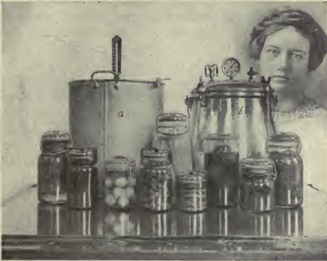
Two types of canning outfits: (a) the water seal; (b) the aluminum steam pressure type, used by a canning club girl.
