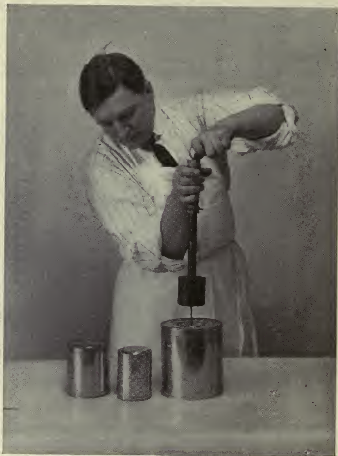
Capping iron, showing position of hand and upright rod. Also how iron is applied to solder hemmed cap.
