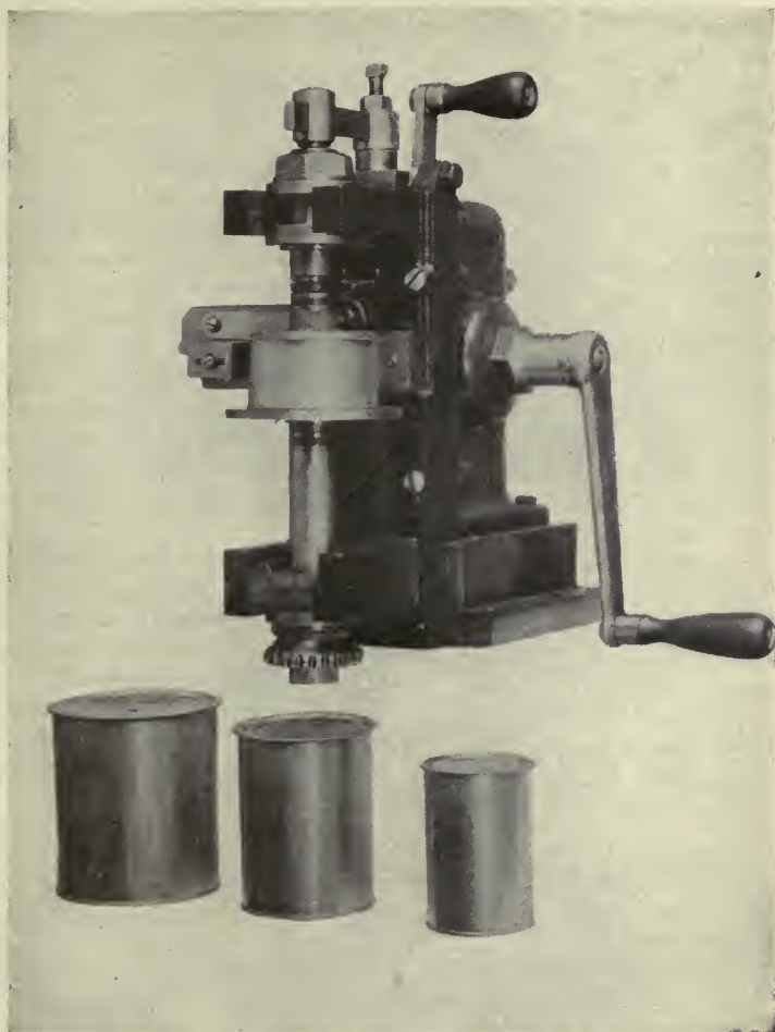
Automatic can sealing machine, seals without heat or solder. Sold, or rented by the year, to clubs and individual growers.
