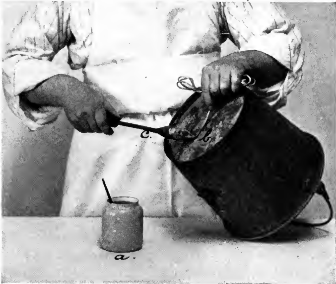
Repairing leak in water-bucket.
