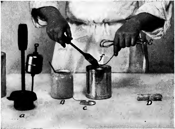
(A) Self-heating capping iron. (B) Flux jar and brush. (C) Solder-hemmed cap. (D) Ammonia bar for cleaning irons. (E) Wire solder. (F) Tipping copper and method of application.
