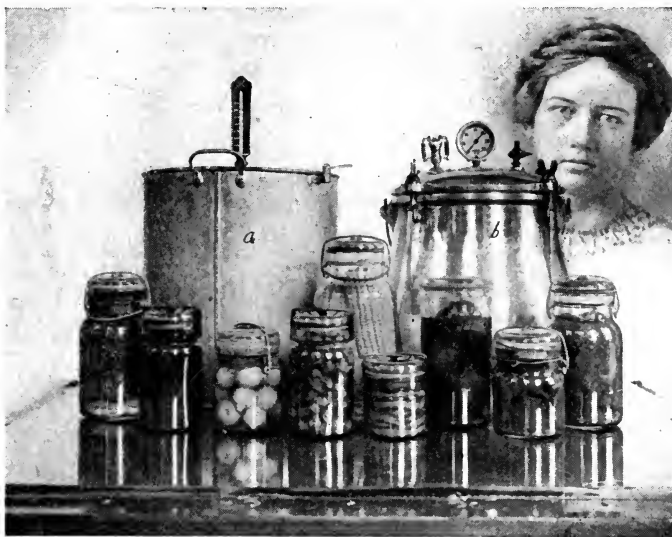
Two types of canning outfits: (a) the water seal; (b) the aluminum steam pressure type, used by a canning club girl.
