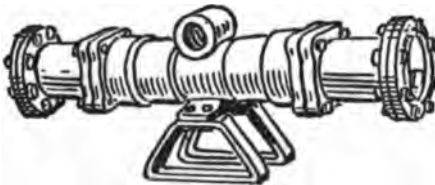
Fig. 245. Double Expansion Joint, Showing Method of Anchoring.
