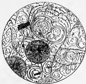
Fig. 42. — Altered Spherulitic Obsidian ("Pyromeride"). Wuenheim, Vosges. \times 7 . Various types of perlitic structure are seen in the devitrified but once glassy matrix.
