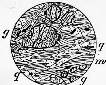
Fig 43.—Mica-Schist. Saxony. \times 7 . g , Garnet, pale pink, and showing signs of cleavage. m , Colourless Mica, bent and drawn out in the direction of the foliation-layers. q , Quartz, granular, and often elongated parallel to the foliation-layers.
