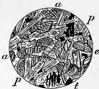
Fig. 29.—Altered Dolerite (Diabase). Mynydd-y-Gader, Cader Idris, N. Wales. \times 24 . a , Characteristic pale-brown augite. e , Almost colourless epidote, associated with pale chloritic areas, in which it crystallises out, giving elongated sections. p , Prismatic plagioclase. t , Titanite iron ore.
