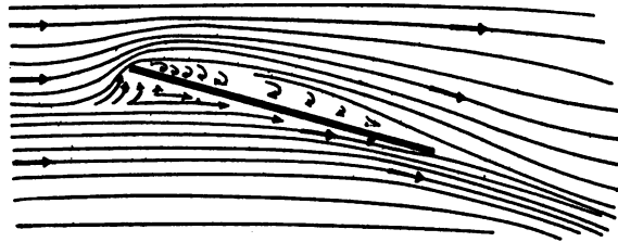
Fig. 5. Flow of air past oblique plane, showing turbulent region back of entering edge and the downward deflection of air after leaving the plane.
