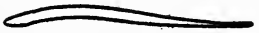
Fig. 18. Wing with reversed curvature toward trailing edge for increased stability. This is paid for by an increase in wing-resistance and a decrease in lift.
