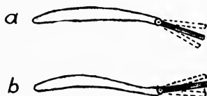
Fig. 11. Section of wing with wing-flap or aileron. In (a) the wing-tip and aileron normally have positive incidence; in (b) they are up-turned and have negative incidence.
