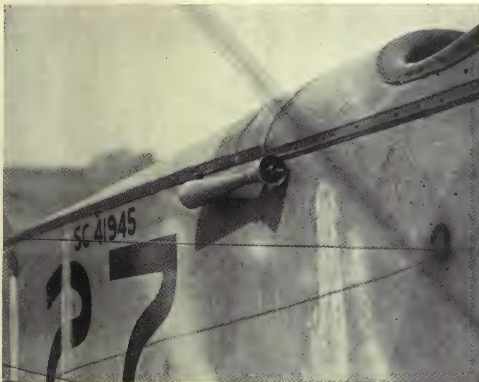
FIG. 55.—Venturi tube on side of plane.
