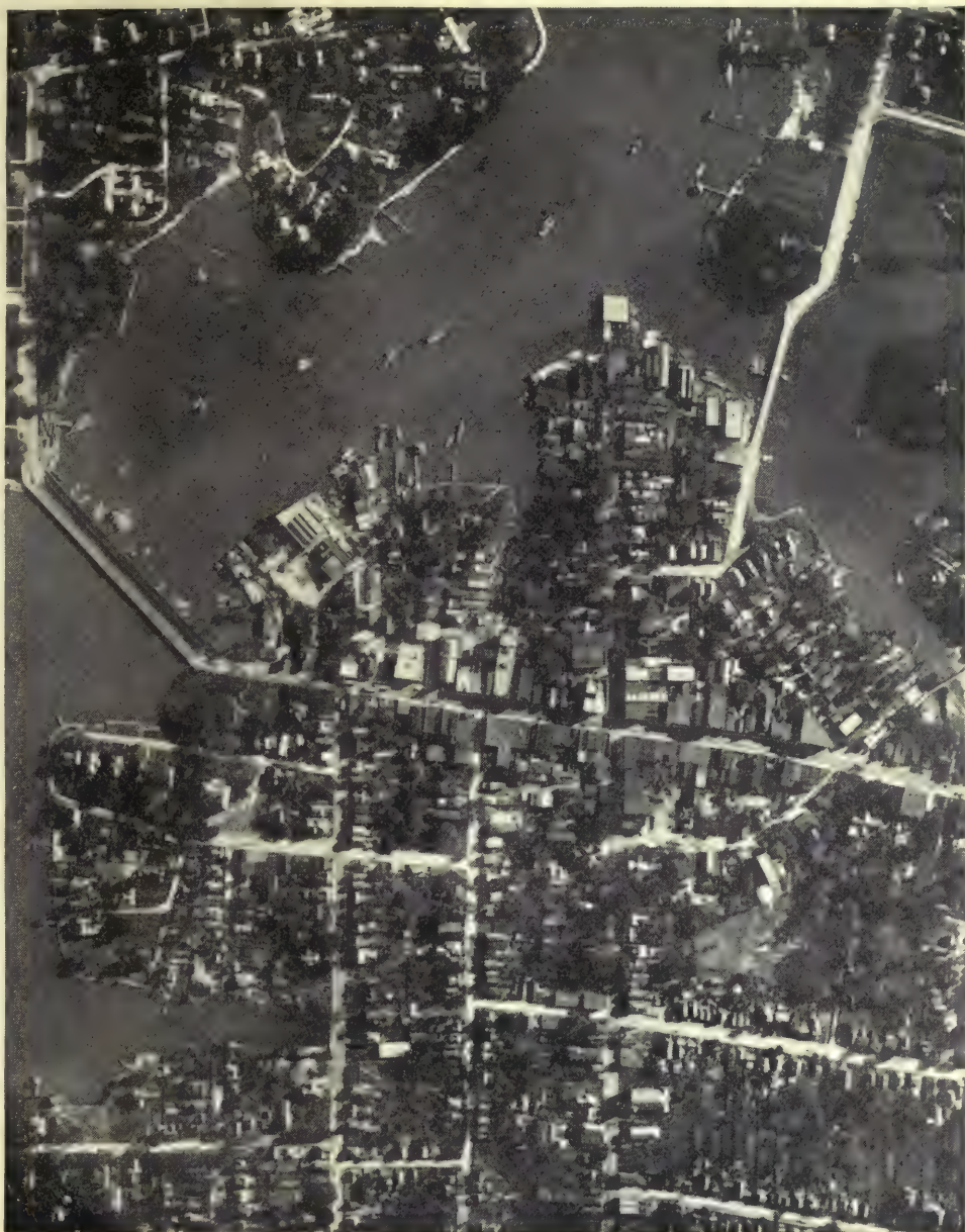
FIG. 202.—Business section of Hampton, Virginia. A survey made by a single instantaneous exposure.
