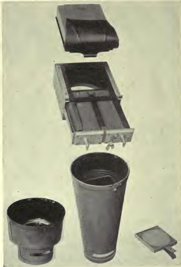
FIG. 44.—U. S. hand-operated aerial camera (type M) with 10 and 20 inch cones.
