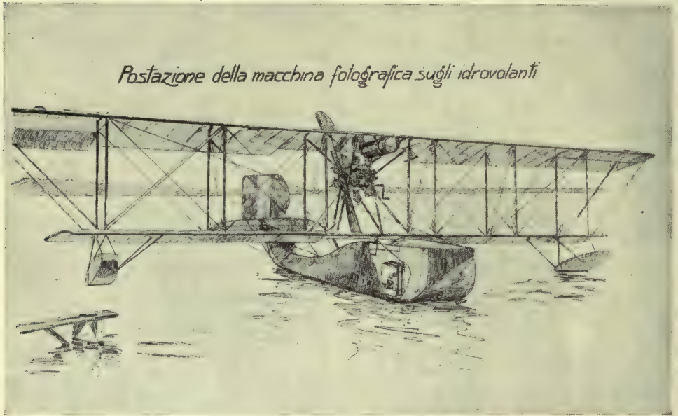
FIG. 187.—Italian flying boat with camera mounted on the floor.
