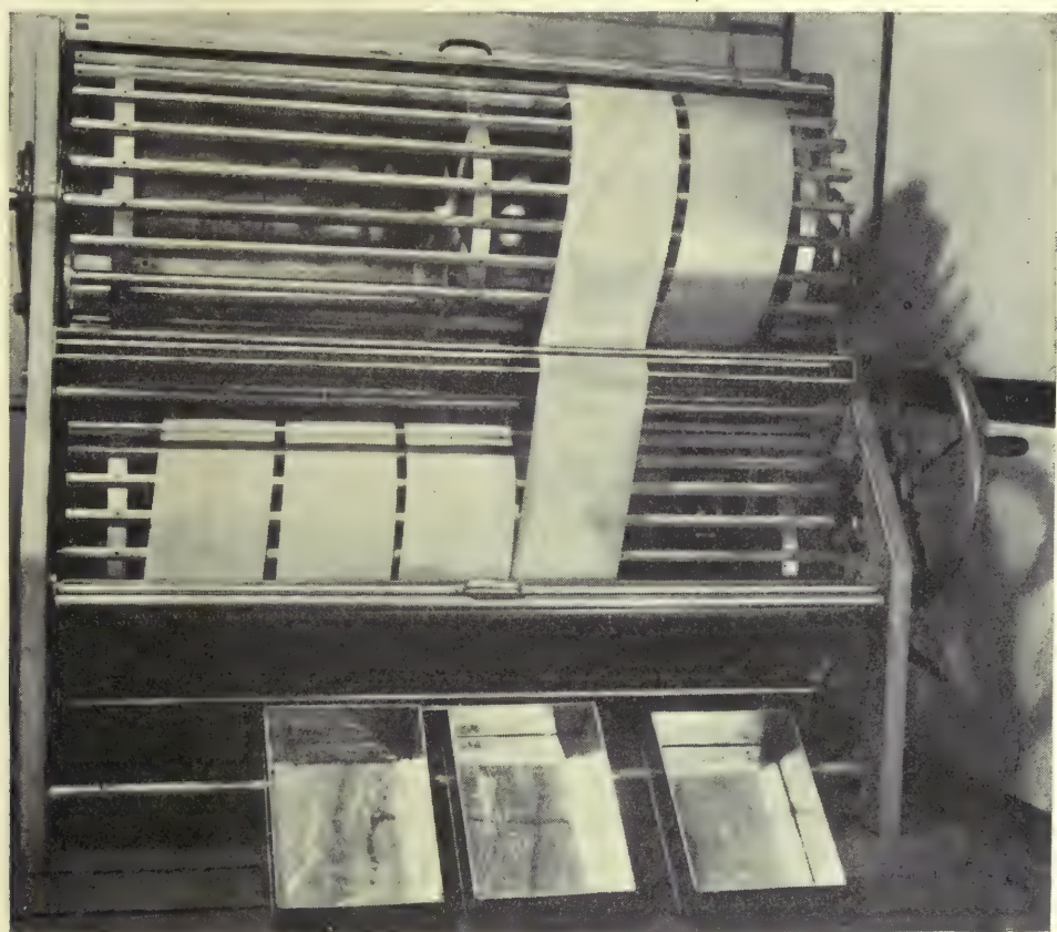
FIG. 117.—U. S. Air Service film developing machine for film 24 centimeters wide.
