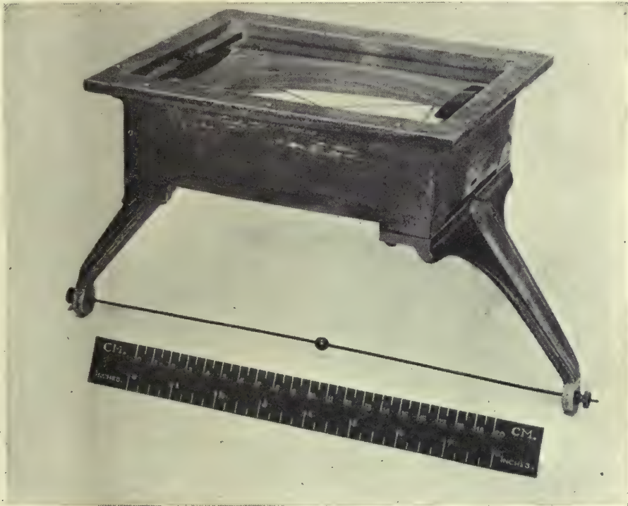
FIG. 73.—Negative lens and mount, side view.
