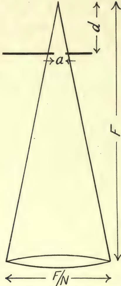
FIG. 21.—Calculation of focal plane shutter efficiency.
