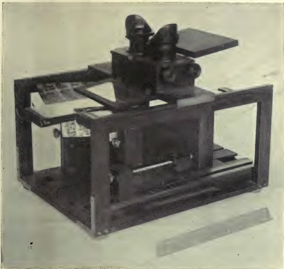
FIG. 154.—Schweissguth stereoscope, used for selecting portions of prints to be mounted.
