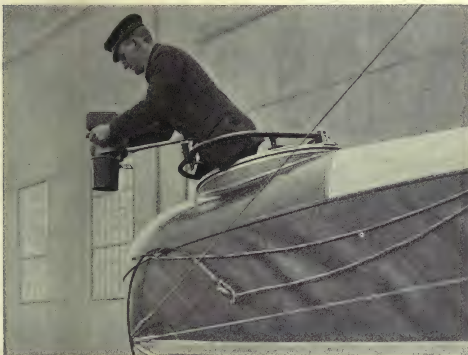
FIG. 186.—Camera mounted in bracket from forward cockpit of flying boat. British official photograph.
