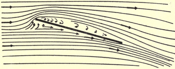
Fig. 5. Flow of air past oblique plane, showing turbulent region back of entering edge and the downward deflection of air after leaving the plane.
