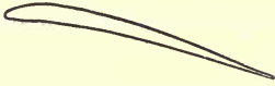
Fig. 15. Wing with high camber, suitable for big lift and slow speed, when flown at large angles of incidence as shown.
