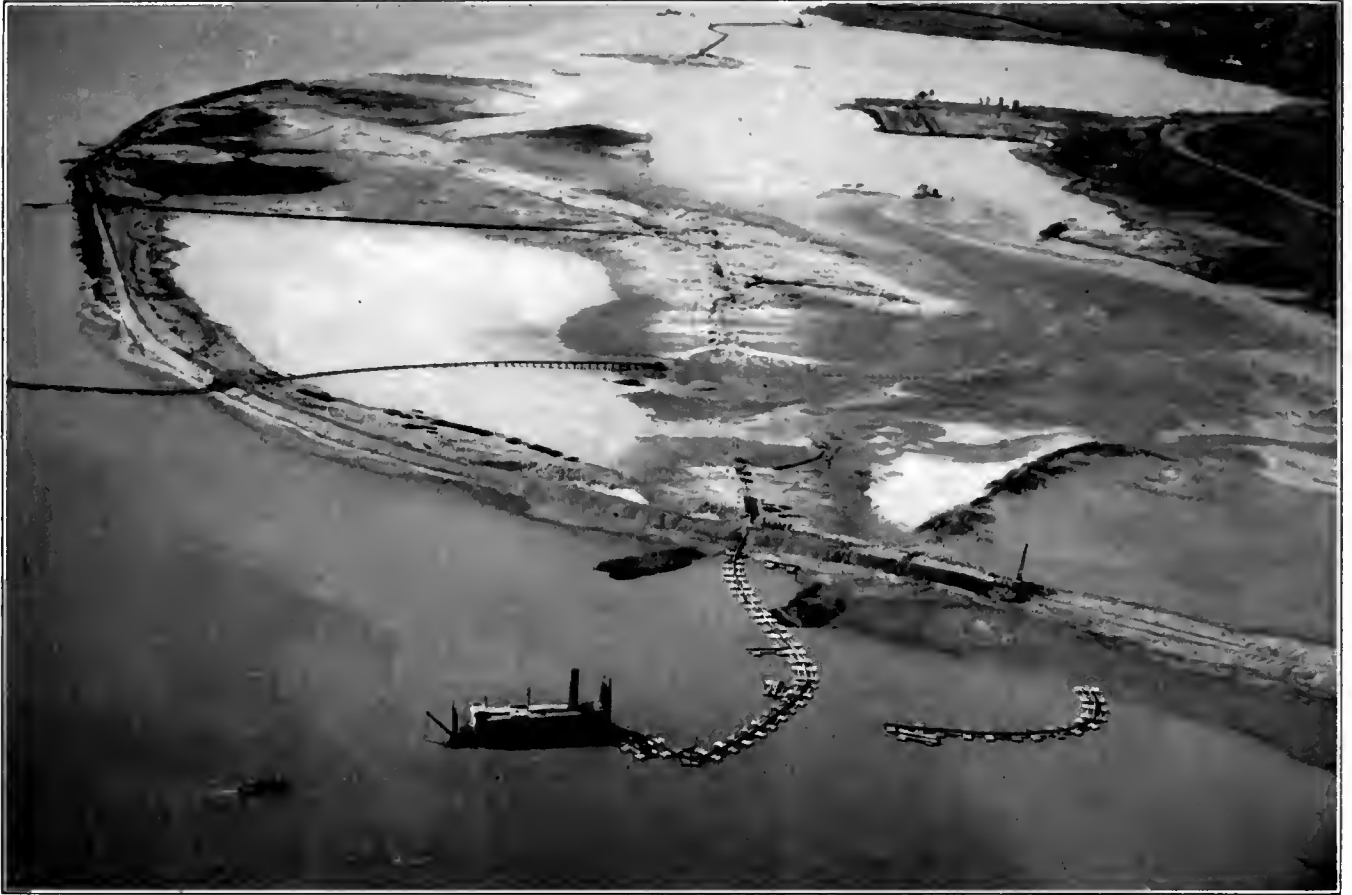
FIGURE 2. AERIAL VIEW OF FILL BEING PUMPED ONTO AIRFIELD AREA
