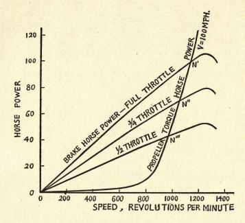
Fig. 49. Speed N', N'' and N''' and corresponding power, for particular engine and propeller, determined for three different amounts of engine throttle, when velocity is 100 MPH.
