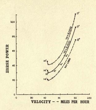
Fig. 40. Variation of required power with velocity. The three curves show effect of changing weight (W = 1000, 2000 and 3000 lbs.) when loading is kept constant (W/S = 6); parasite resistance =  $0.04 V^2$ .
