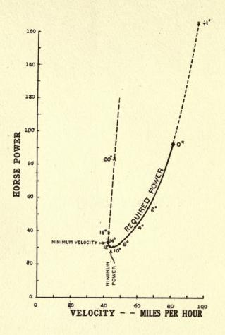
Fig. 39. Required power at different velocities, when W = 2000 lbs.; W/S = 6; parasite resistance  $= 0.04 V^2$ .
