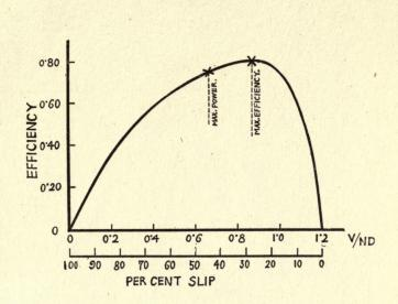
Fig. 55. Propeller efficiency for different values of V/ND. Efficiency is equal to thrust horse power divided by torque horse power; see Fig. 52. Pitch ratio, 0.9. Values for V, N or D are not fixed.
