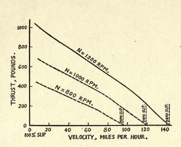
Fig. 51. Variation of thrust with velocity, for a particular propeller, when driven at constant speed. Pitch ratio 0.9, diameter 8' 9''.
