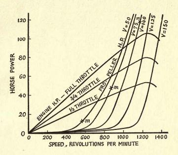
Fig. 50. Curves for engine brake horse power for different amounts of throttle and propeller torque horse power for different velocities. Intersections determines speed and power for each velocity and amount of throttle. Maximum efficiency at m.
