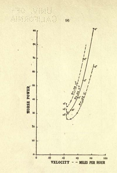
Fig. 43. Variation of required power with velocity. The three curves show effect of changing parasite resistance  $(R = 0.02 V^2, R = 0.04 V^2)$  and  $R = 0.06 V^2$ ; weight and loading constant (W = 2000 lbs.; W/S = 6).
