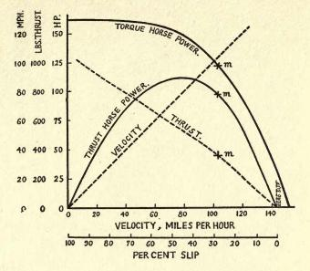
Fig. 52. Variation of thrust horse power with velocity for a particular propeller when driven at 1200 R. P. M. Dotted curves show thrust and velocity. The upper curve, reproduced from Fig. 47, shows torque horse power.
