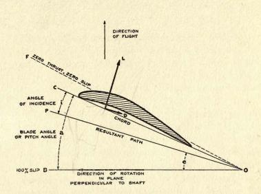
Fig. 60. Particular section of propeller blade at distance of r from center of shaft, showing the behavior of a propeller blade as an aerofoil, attacking the air at an angle of incidence i.
