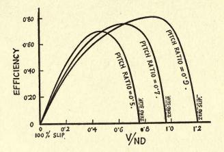
Fig. 56. Efficiency of three similar propellers with different pitch ratios.
