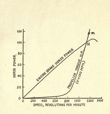
Fig. 48. Speed N and power, of particular engine and propeller, determined by intersection of curves for engine brake horse power and propeller torque horse power.
