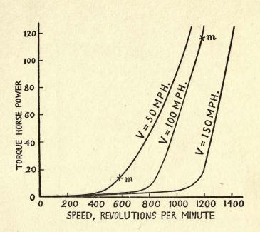
Fig. 46. Torque horse power required to drive a particular propeller at different speeds (revolutions per minute) when travelling through the air at 50, 100 and 150 M P H., at ground level. Propeller diameter, 8' 9"; pitch ratio, 0.9. Maximum propeller efficiency is at m.
