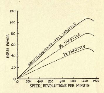
Fig. 44. Variation of brake horse power of a typical gas engine with speed. Dotted curves show reduction of power by throttle control.
