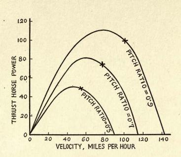
Fig. 57. Thrust horse power of three similar propellers with different pitch ratios. Point of maximum efficiency is marked by x.
