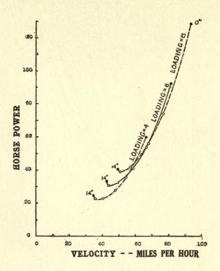
Fig. 41. Variation of required power with velocity. The three curves show effect of changing loading (W/S = 4, 6 and 8) when weight is kept constant (W = 2000 lbs.); parasite resistance =  $0.04 V^2$ .
