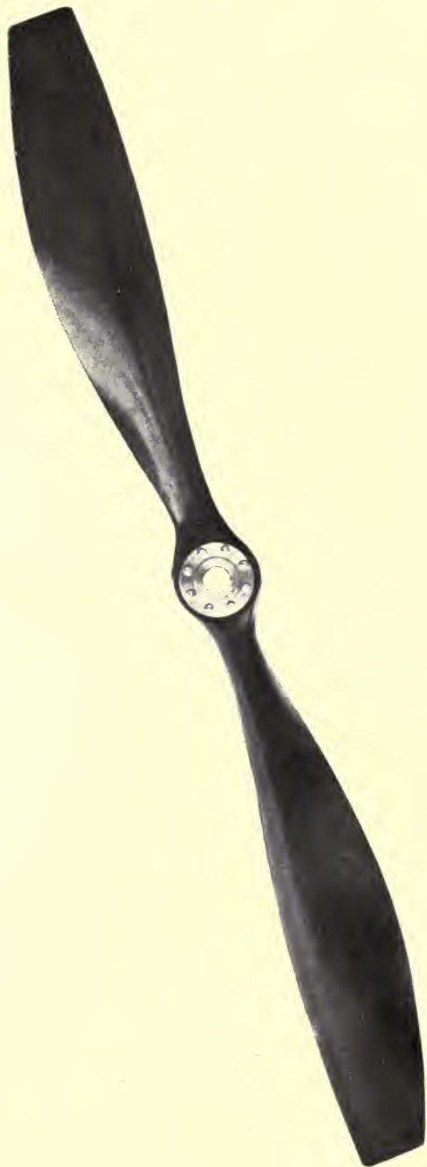
TWO-BLADED AIR-SCREW DESIGNED BY THE AUTHOR FOR 60 HP. LE RHÔNE AEROPLANE ENGINE.
