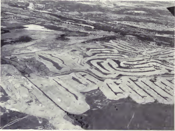
FIG. 81. Placer mining near Folsom, California, in the foot-hills of the Sierra Nevada. The view shows the dumps of gravel left by the dredges.
