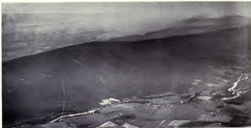
FIG. 22. An eroded pitching anticline. This anticline is pitching toward the left. The two ridges, formed by the limbs of the anticline, converge and join to form a single ridge.
