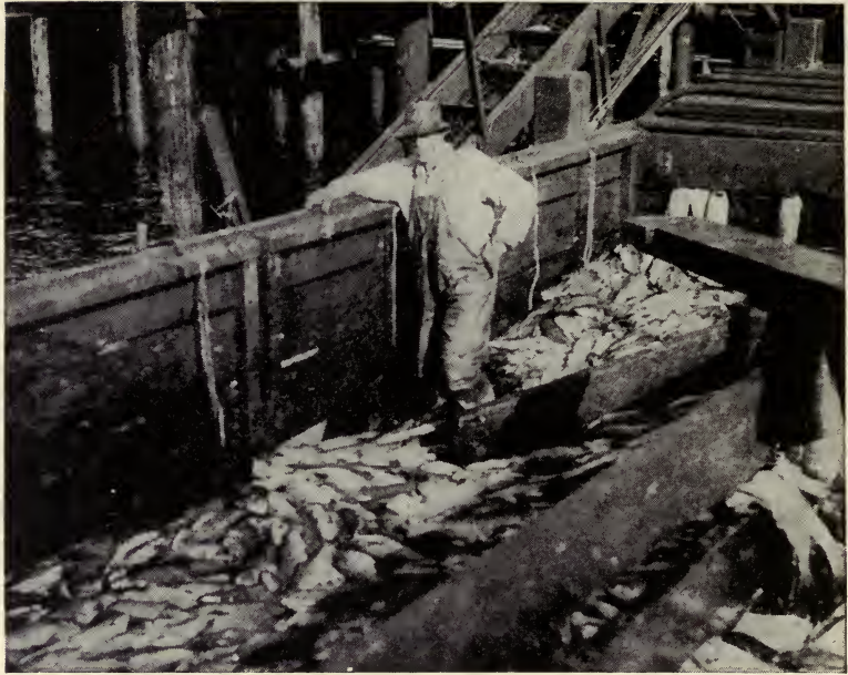
Unloading salmon from a scow at Ketchikan, and hoisting the fish into cannery bins by means of an escalator. (U.S. Fish and Wildlife Service.)
