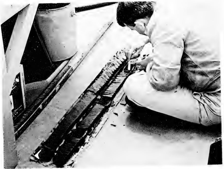
Fig. 30 Core being studied on deck of Velero III
