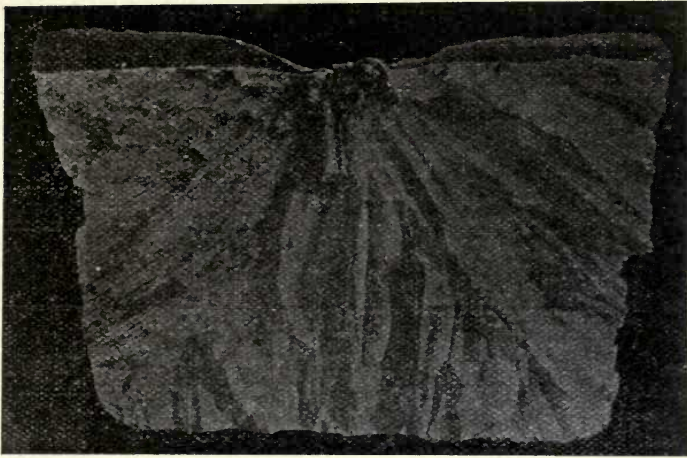
FIG. 59.—FRACTURE OF BRASS CONTAINING .05 PER CENT. OF ANTIMONY.
