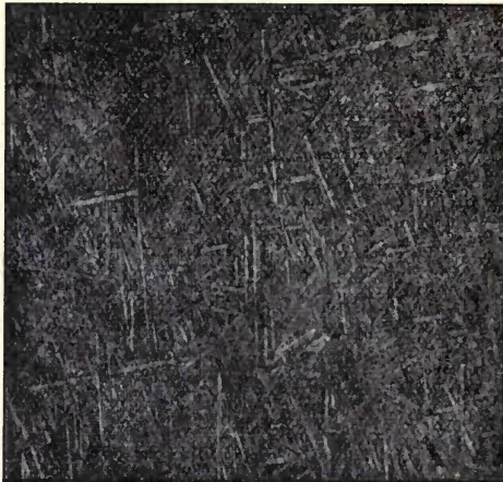
FIG. 91. Aluminium bronze, 10 per cent. aluminium. Heated to 900°C. and quenched \times 75 .
