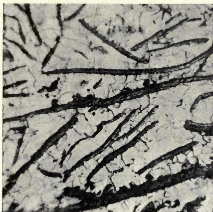
FIG. 36.—CRYSTALS OF GRAPHITE SEPARATED IN A GROUND MASS OF FERRITE.
