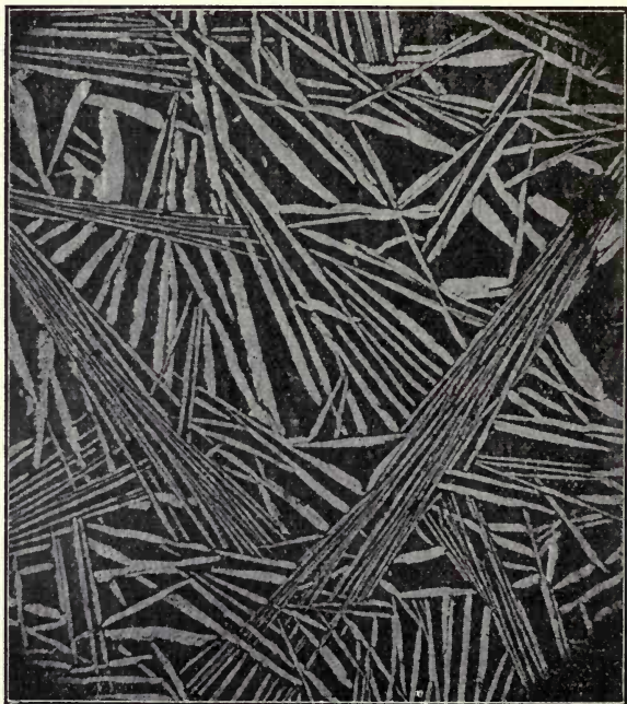
FIG. 82.—PHOSPHOR TIN, 9.78 PER CENT. PHOSPHORUS. MAGNIFIED 40 DIAMETERS. VERTICAL ILLUMINATION.
