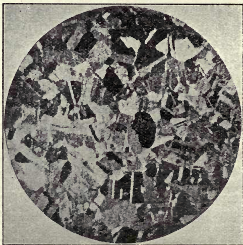
FIG. 41.—BRASS AFTER HEATING TO 600° C. (MAGNIFICATION 58 DIAMETERS.)
