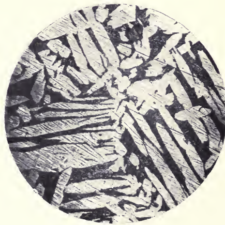
PHOTOGRAPH 30. CUPRO-ALUMINIUM. CAST AND ANNEALED AT 800°. × 225.
