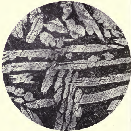
PHOTOGRAPH 4. CUPRO-ALUMINIUM. FORGED AND SUBSEQUENTLY ANNEALED AT 300°. × 225.
