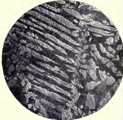
PHOTOGRAPH 12. CUPRO-ALUMINIUM. FORGED AND SUBSEQUENTLY QUENCHED FROM 600°. × 225.
