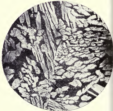
PHOTOGRAPH 8. CUPRO-ALUMINIUM. FORGED AND SUBSEQUENTLY ANNEALED AT 900°. × 225.
