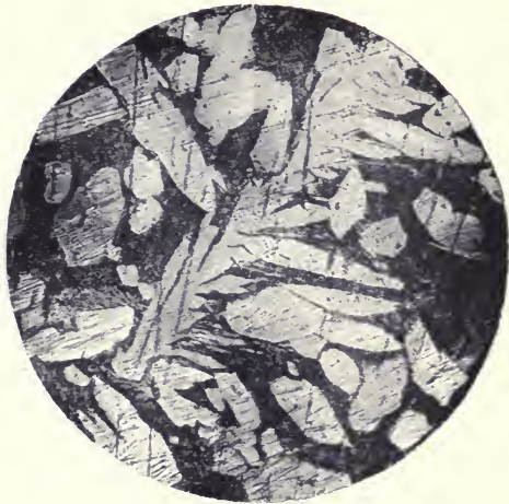
PHOTOGRAPH 28. CUPRO-ALUMINIUM. AS CAST. × 225.
