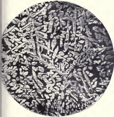
PHOTOGRAPH 27. CUPRO-ALUMINIUM. AS CAST. × 60.
