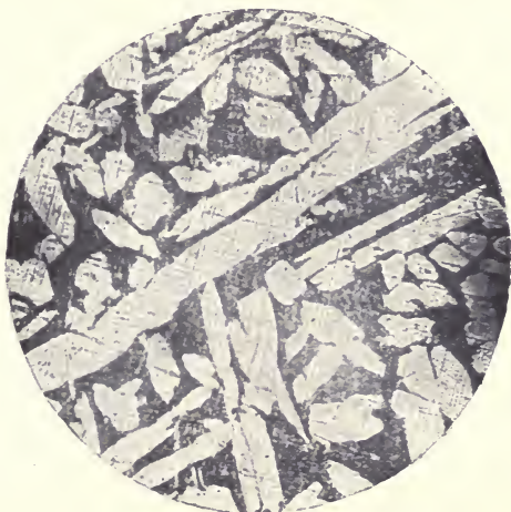
PHOTOGRAPH 32. CUPRO-ALUMINIUM. CAST AND ANNEALED AT 900^{\circ} . \times 225 .
