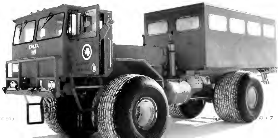
This delta is a twenty-eight-year-old Navy vehicle that can transport up to twenty passengers over the ice.
