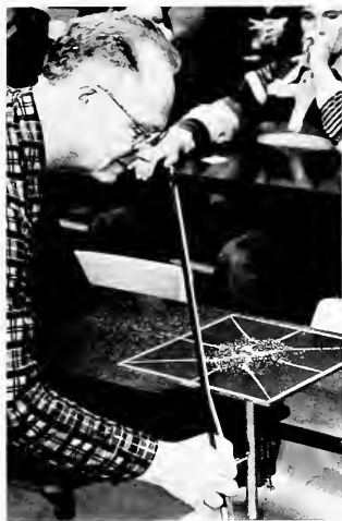
Physicist Clifton Bob Clark creates visible sound patterns using blasting powder on a quarter-inch brass plate.
