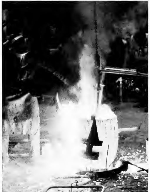
Herk van Tongeren de-gasses the molten brnze and (at far left) Richard Kallath '68 MFA, a member of the art faculty, operates the hoist. At right Herk stabilizes the crucible.
