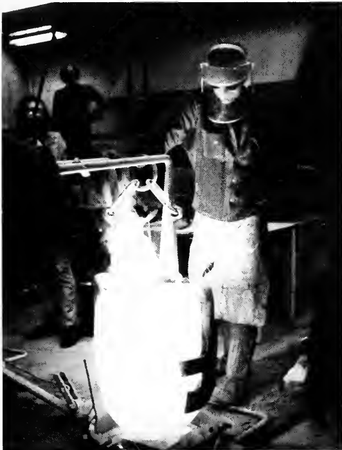
Herk van Tongeren de-gasses the molten brnze and (at far left) Richard Kallath '68 MFA, a member of the art faculty, operates the hoist. At right Herk stabilizes the crucible.
