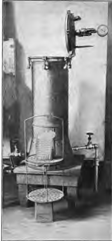
FIG. 10. Autoclave fitted with steam connections
