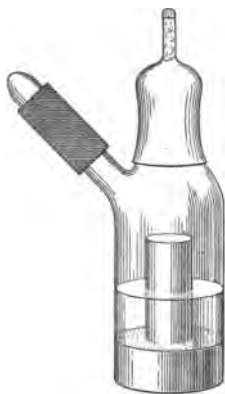
FIG. 37. Gypsum block in a Hansen flask
