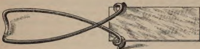
FIG. 9.—KIRKBRIDE FORCEPS FOR HOLDING SLIDES.
