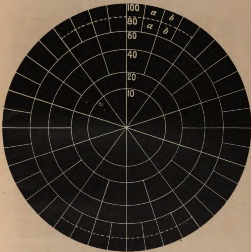
JEFFER'S PLATE (Bausch and Lomb). FOR COUNTING COLONIES OF BACTERIA ON CIRCULAR PLATES. THE AREA OF EACH DIVISION IS ONE SQUARE CENTIMETER.
