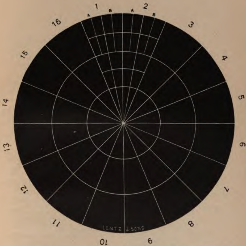
PLATE FOR COUNTING COLONIES OF BACTERIA IN PETRI DISHES.
