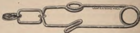
FIG. 8.—STEWART FORCEPS FOR COVER-GLASSES.
