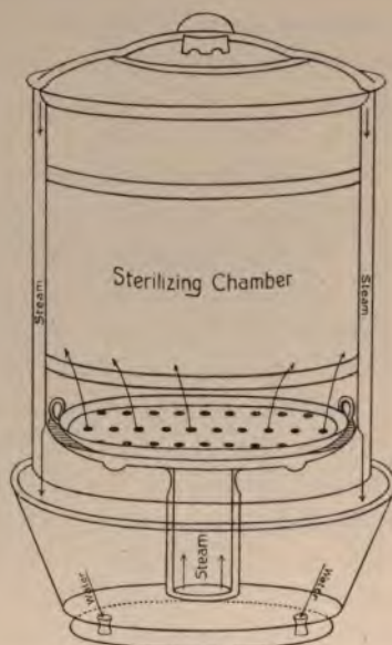
FIG 12.—DIAGRAM OF THE ARNOLD STEAM STERILIZER.
