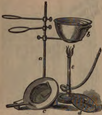
a , Retort Stand; b , Water Bath; c & d , Piffard's Water Oven; e , Bunsen Burner.
