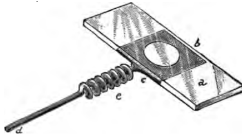
FIG. 16.—Slide for heating: a , slide; b , copper plate; c , arm over which the spiral wire ( d ) is slipped
