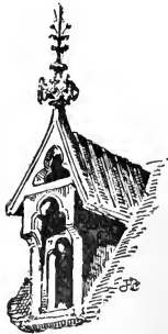
Dormer Window on Roof.
