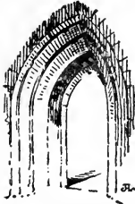
Perpendicular Shaft and Arch Mouldings.
