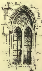
Window and Dripstone.
