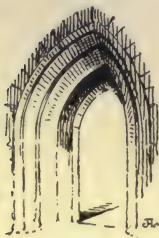
Perpendicular Shaft and Arch Mouldings.
