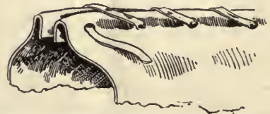
Fig. 4.—Method of Sewing the Leather Covers.
