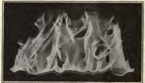
FIG. 3. FLAMING DISCHARGE OF 250,000 VOLT TRANSFORMER.—By Percival E. Fansler.
