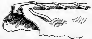
Fig. 4.—Method of Sewing the Leather Covers.
