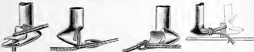
BEHEL'S TYING BILL—FORMING THE KNOT.
