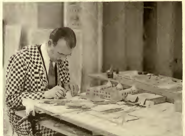
No. 2. Gluing and fitting the side elevations, cut from the mounted Whatman paper, together.
