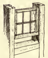
Crude beginning of the sliding sash
