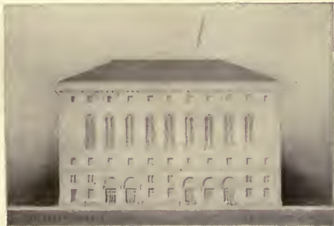
Elevation of the original scheme—which contemplated facing the old brick structure with marble.
