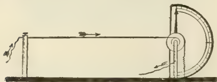
FIG. 7.—Simple Illustrative Model of Hot-wire Amperemeter.
