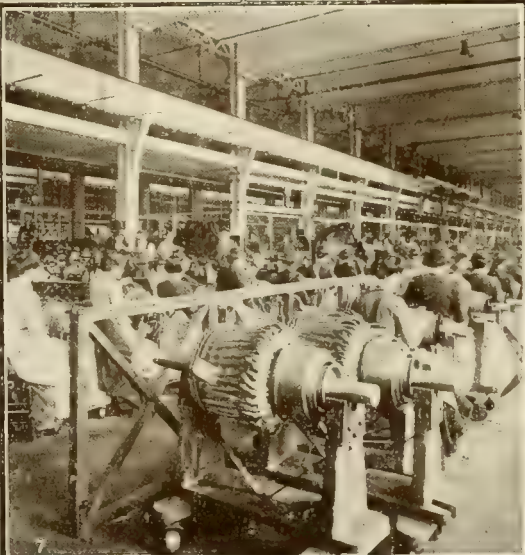
1 Heavy Construction Work in the Erecting Shops. 2 A Section of the Winding Department where Small Coils are Made. 3 Assembling Armature Cores. 4 Mounting Large Transformers. 5 Mica-Splitting Machine. 6 650 Horse Power Gas Engine Generating-Set in the Power Station. 7 Connecting Street Railway Armatures. INTERIOR VIEWS IN THE WORKS OF THE WESTINGHOUSE ELECTRIC AND MANUFACTURING COMPANY.
