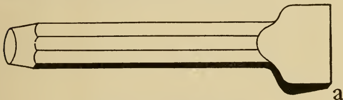
Fig. 73. The pitching tool.
