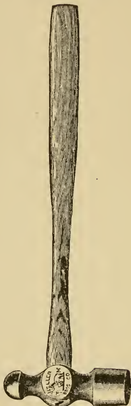
Figure 74 Heller Bros'. Hammer for Horseshoers
