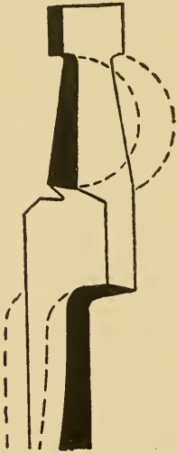
illustrating how jaws are forged and bent to shape.
