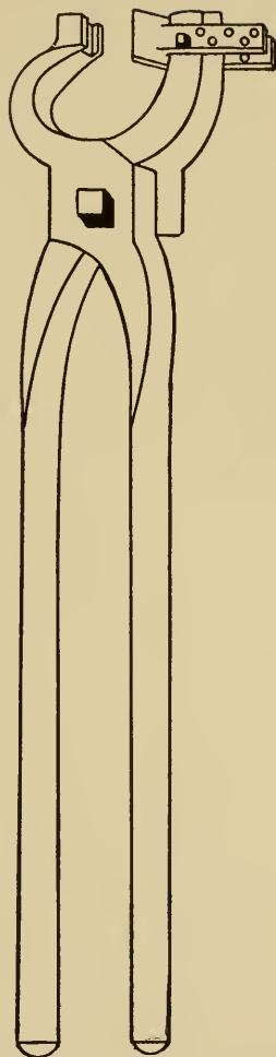
Fig. 4. Adjustable tongs regulated for holding largest size.
