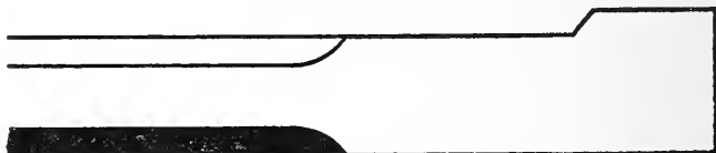
Fig. 99. Showing steel upset to forge heel on punch bar.
