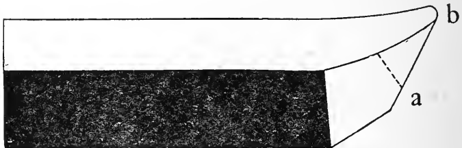
Fig. 47. Heavy roughing tool.
