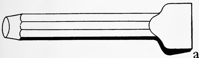
Fig. 73. The pitching tool.
