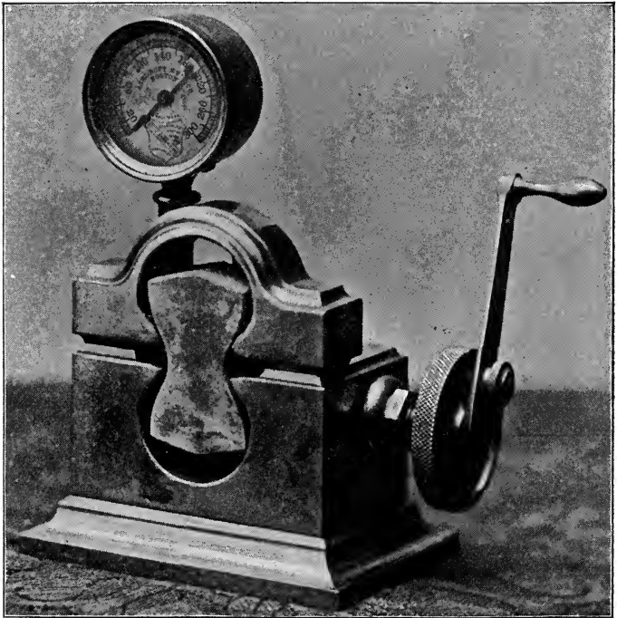
CUMMING'S HYDROSTATIC CEMENT TESTER, CAPACITY 300 POUNDS.
