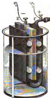
FIG. 5.—Cell of Wollaston's Battery.
