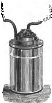
FIG. 7.—Cell of Daniell's Battery.
